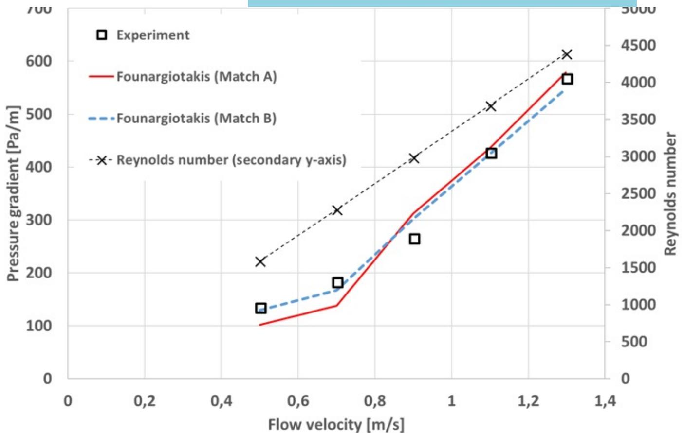
Figure 3. Pressure gradient is plotted for the experimental data and for modelling with fluid parameters based on the curve matches A and B. The corresponding Reynolds numbers are also included.
