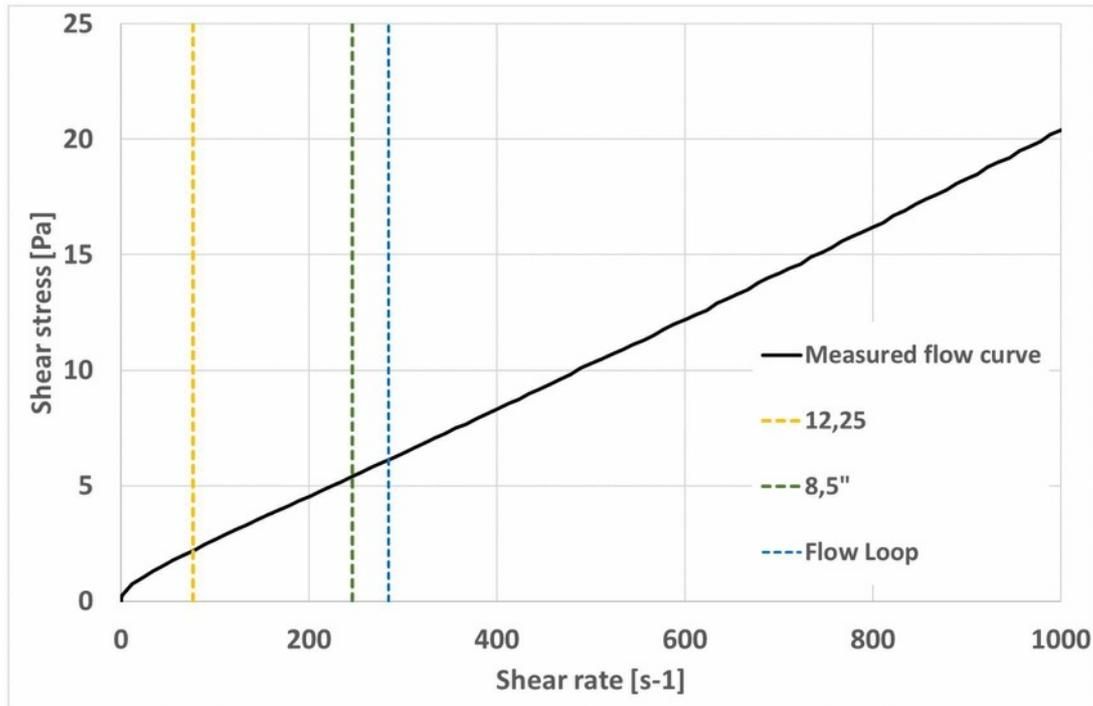
Figure 1. Flow curve is plotted for measurements according to API standards. Normal maximum shear rates for operations and flow loop are included.
